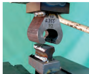
After testing, failure through deformation
