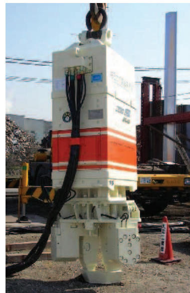
Vibratory hammer equipped with clamp for hat-type sheet pile 900
